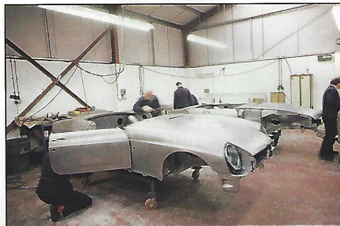
An RV8 bodyshell being finished at the BMH Faringdon works; these really were hand-built cars, every step of the way. (Classic & Sports Car)
