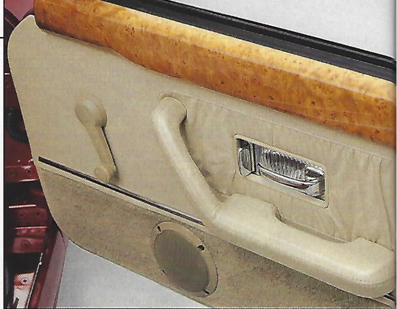
The interior door catch is as on Jaguars, and the armrest is borrowed from another car too. Manual-only windows were criticised at the time
