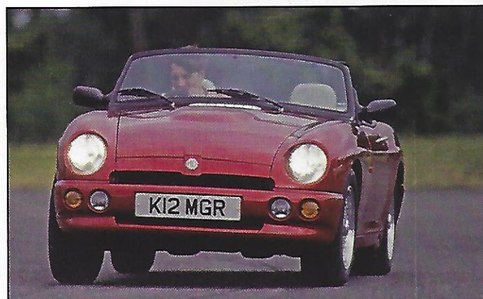
The 3.9-litre Rover V8 develops 190bhp, making the RV8 good for 136mph and 0-60mph in 6.9 seconds, according to the Autocar test
