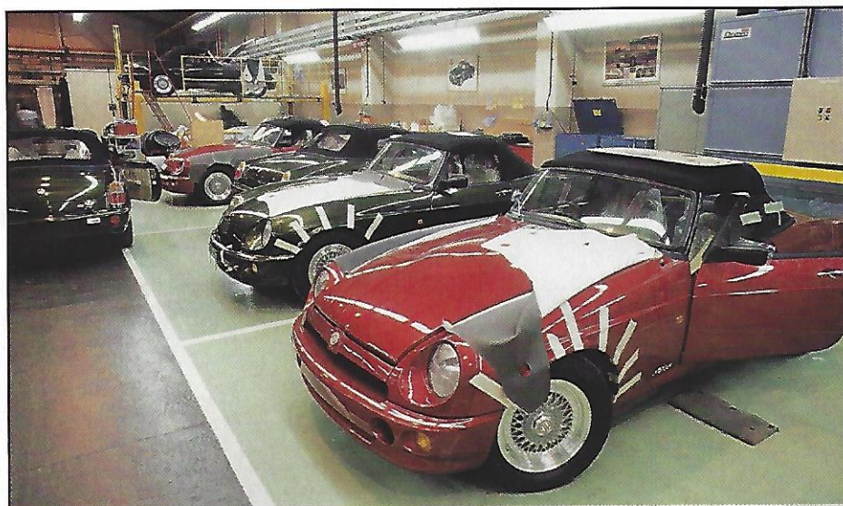
Final adjustments being carried out; in the foreground are two Japanese-market cars, wheelarch extensions taped in place. (Classic & Sports Car)
